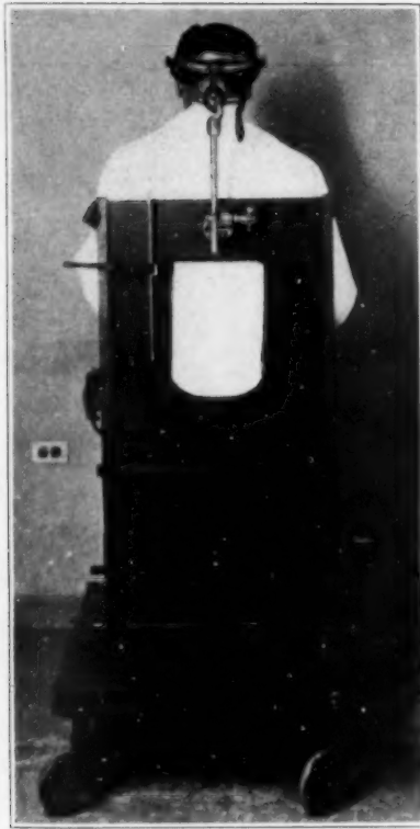
Fig. 5.—Back view of chair, showing head rest in position, manometer and holder.
